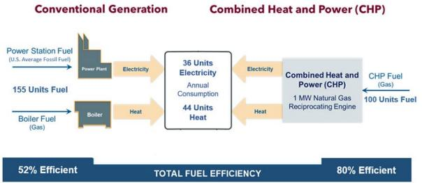
This is an example of a typical CHP system. To produce 80 units of electricity and useful thermal energy, the conventional system uses 155 units of energy inputs—an overall efficiency of 52 percent. However, the CHP system needs only 100 units of energy inputs to produce the 80 units of electricity and useful thermal energy, resulting in a total system efficiency of 80 percent.
